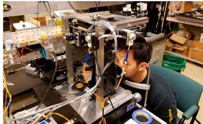
Postdoctoral researcher Shijun Sung scanning his cornea with a prototype THz imaging system. The system scans the imaging beam while the patient's head stays fixed using standard ophthalmic chin and forehead rests.
