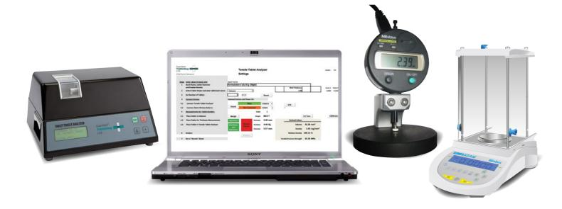
balance to provide an integrated assessment of tablet properties. The system utilises a 4-figure analytical balance and digital micrometer to automatically capture and send thickness, weight and fracture data to the computer in real time. Dynamic powder compaction analysis can also be carried out using the unique Gamlen punch position and force measurement combination.
