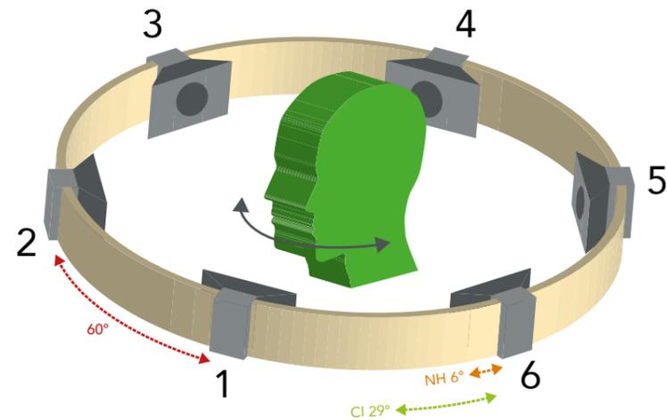
Figure 1. Schematic illustration of the experimental apparatus. Speakers are spaced 60° apart. Root-mean-squared (RMS) localization error in the frontal hemifield for normal hearing listeners for all broadband stimuli was measured, using many more loudspeakers than six, as approximately 6°. RMS error for cochlear implant listeners for high-frequency stimuli is approximately 29°.
