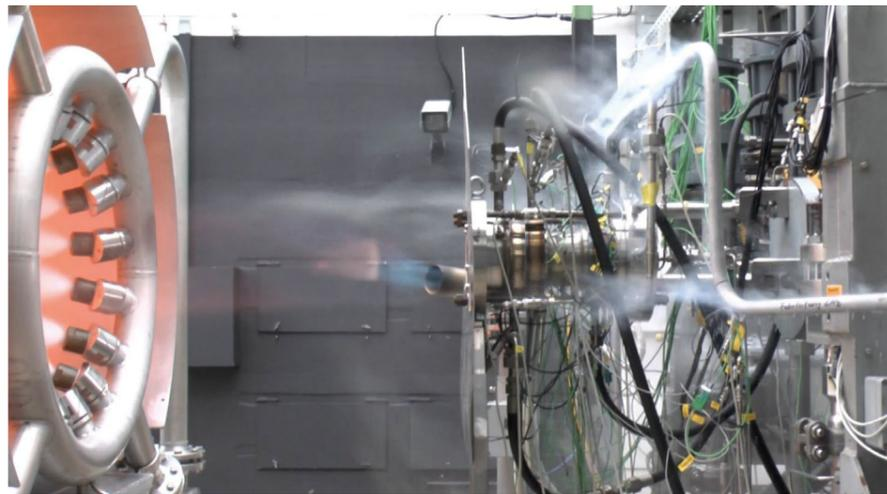
BKD during a test at the P8 test facility, where self-excited flame dynamics are measured with fibre-optical probes. A modified version of BKD with an optical access window is currently in testing.
