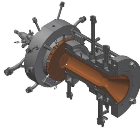
A conceptual illustration of the inside of the BKH experimental combustor with a rectangular cross-section, siren in the upper wall for acoustic forcing, and optical access windows. On the right is a numerical simulation of the cryogenic flames and flow field inside BKH. This kind of result is compared to experimental data from BKH to validate the simulation method.
