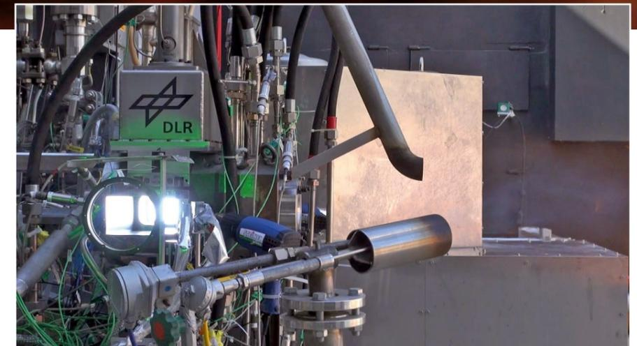
BKH during a test at the P8 test facility, with siren forcing of the internal combustor acoustics and high-speed imaging of the flame response through the windows in the side walls.
