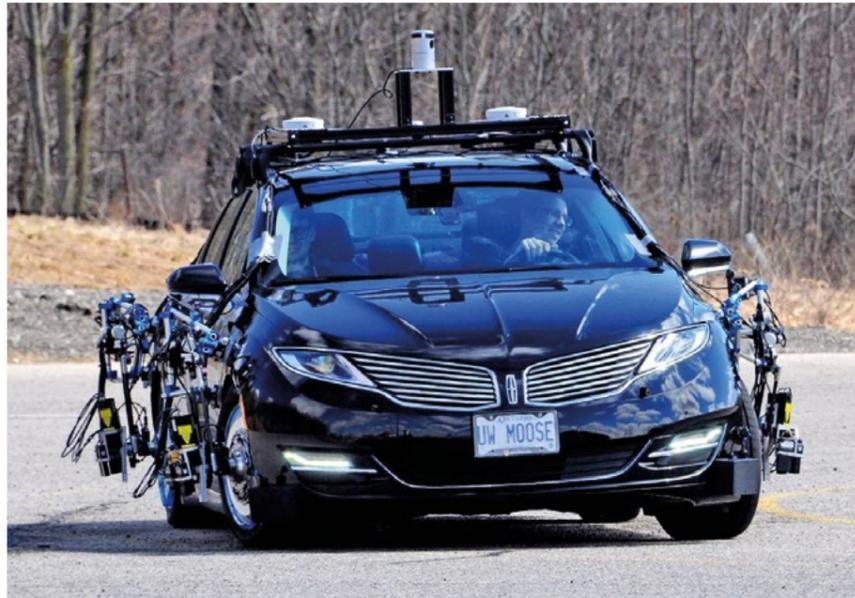
High-speed track testing of the Automoose (or "The Moose", Canada's first autonomous vehicle) with Waterloo's vehicle measurement system.
