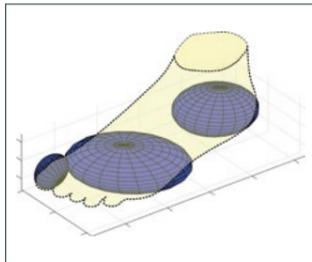
The volumetric contact model to predict foot-ground interaction forces.
