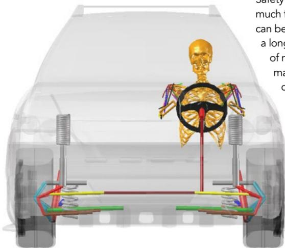
Electric power steering control using biomechatronic model of driver and vehicle.
