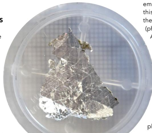
Photograph of a typical hBN crystal
