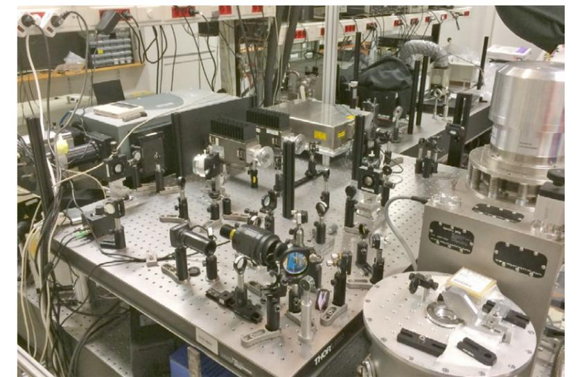
The deep UV microscope with ultimate spatial resolution at 200 nm limited by light diffraction. The low temperature chamber hosting the sample and the microscope objective is on the right of the picture.
