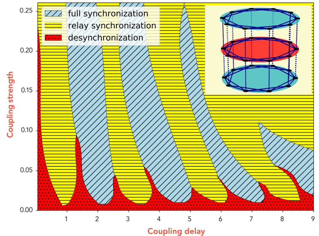
Relay synchronisation 'tongues' in the parameter plane of inter-layer coupling strength and in-layer coupling delay.
