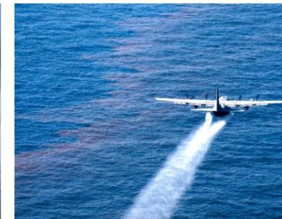
A C-130 Hercules sprays Corexit dispersant onto the affected water.
