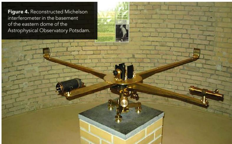
**Figure 4.** Reconstructed Michelson interferometer in the basement of the eastern dome of the Astrophysical Observatory Potsdam.
