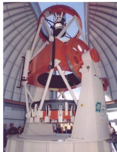
Fig. 6 MOA telescope used to search for exoplanets by gravitational microlensing.
