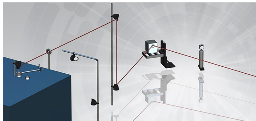
A laser path from the laser on the right (laser not shown) to the mass spectrometer on the left. The laser beam enters the ion trap, bounces off mirrors outside the trap, and exits the mass spectrometer.
