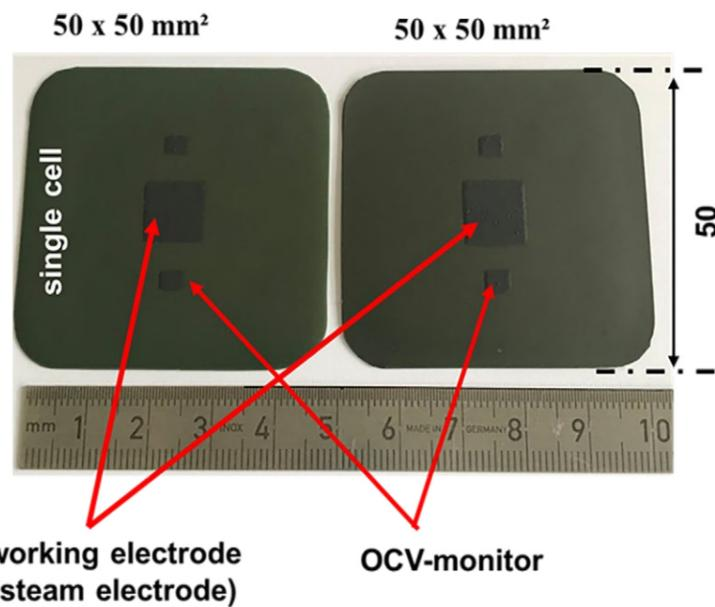
Size of the steam electrode on a single cell.
