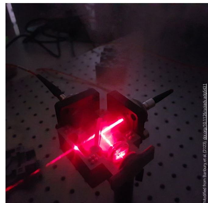
Inside the EyeD Technology: Concurrent optical and Raman paths.
